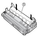
**9** Turn the two levers (1) on the toner cartridge firmly.
